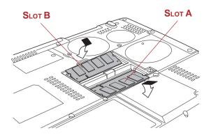
Figure 8-4 Installing the memory module
